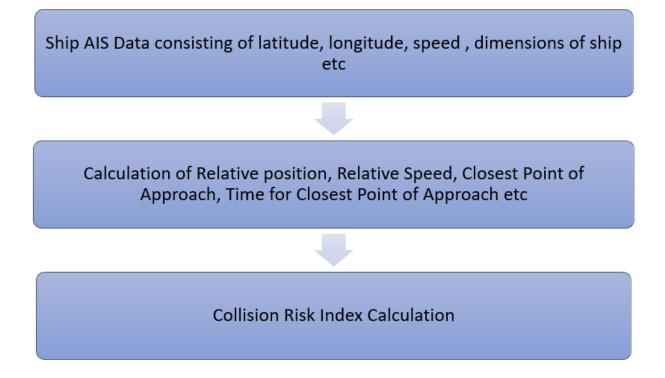
First, the Data from Marine Traffic are used to calculate the position, speed, CPA, and TCPA, and with these parameters being fed in a Machine Learning/Mathematical model, CRI is Calculated, and with this CRI, an alarm is triggered.
